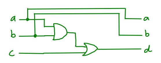
If we can produce a quantum circuit to simulate this gate, quantum circuits are also universal for classical computation
