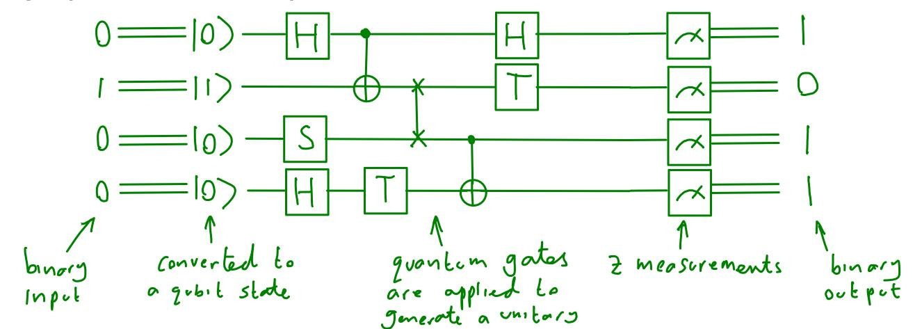
This is a quantum computer, according to the circuit model
